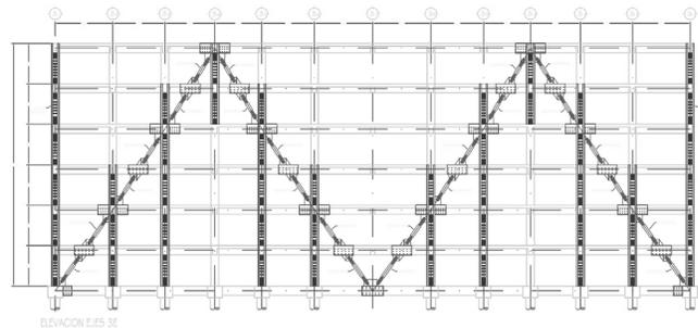
Image 6. BRB alternative in the long side (X) (left), short side (Y) right, columns jacking
