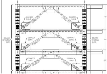
Image 8 Typical arrangement of YRB proposal in the short sense (Y) (left)
