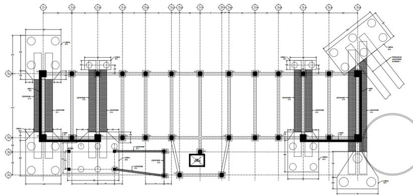
Image 4. Foundations design of the shear wall alternative, 36 piles
