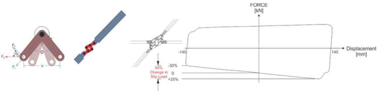
Image 11 Variation in force in rotational mechanisms
