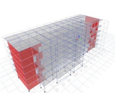
Image 3. Model with shear walls as SFRS
